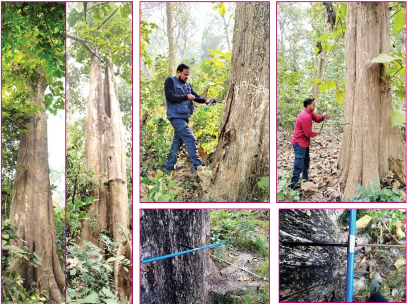
Fig. 7 - Sampling of tree-ring cores (*Tectona grandis*) from Maharajganj District, Uttar Pradesh, using an increment borer.
